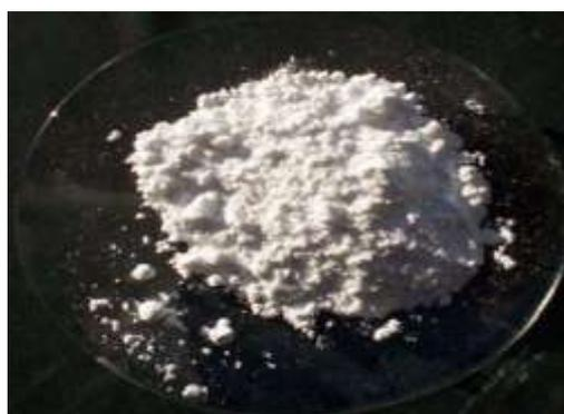
Figure-2. A sample of calcium carbonate ( $\text{CaCO}_3$ ).limestone filler.
